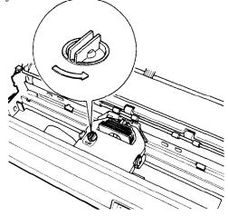
7. Slide the print head from side to side to make sure **that** it moves smoothly. (Do not try to slide the print head by grasping the ribbon cartridge.)
